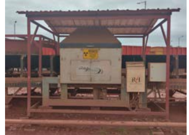
RTI's AllScan cf-252 elemental analyser on site.
